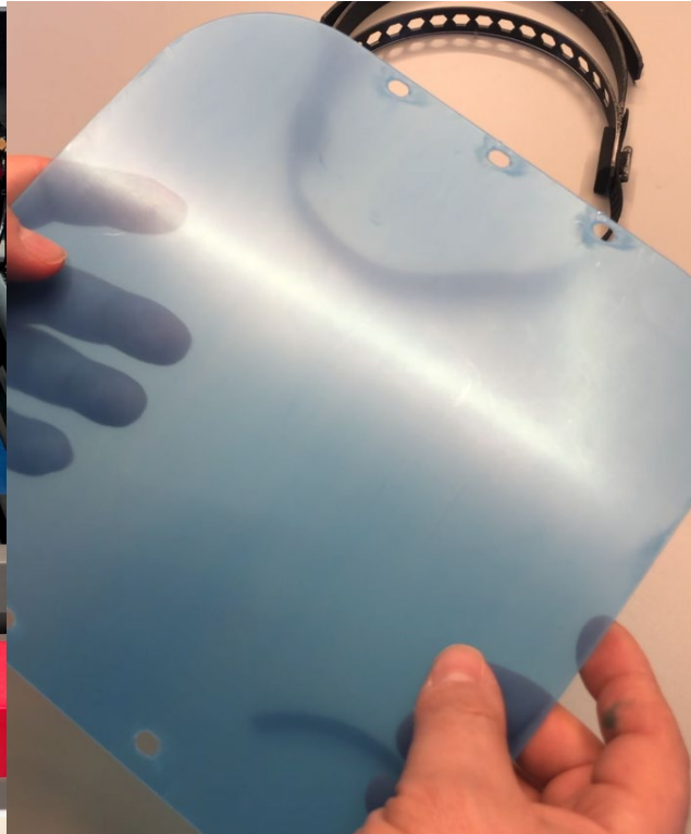
Finished shield laser cut ready to be placed on head band
